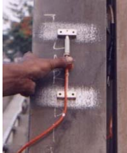
Gambar 10. Vibrating wire accoustic strain gauge.
